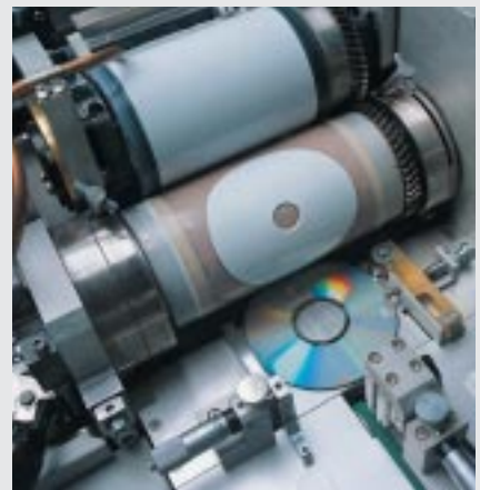
A multi-function white basic unit with UV dryer for applying white primer coating to the discs is placed between the feed unit and the print stations (can be configured for rotary screen printing or flexo print).
