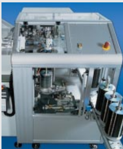
Input handling and code reader with spindle, buffer and feed handling.
