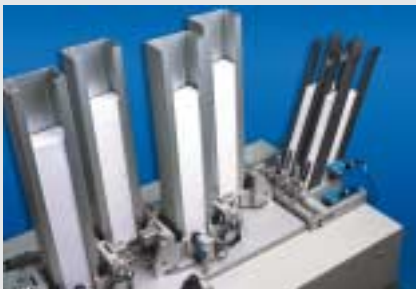
Loading magazine module (right) and four additional card holds for large print runs significantly reduce the need for reloading.
